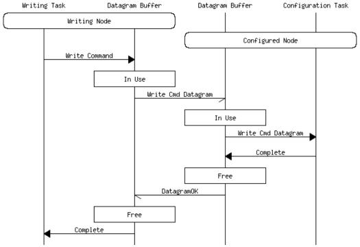
A typical memory write operation. The Write Command and data are carried to the node being configured in a single datagram. Since the write operation succeeds immediately, the only reply needed is the datagram reply.
